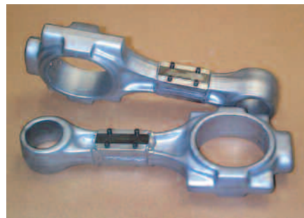
FIGURE 11-6 Almen Strip Mounting Fixture
