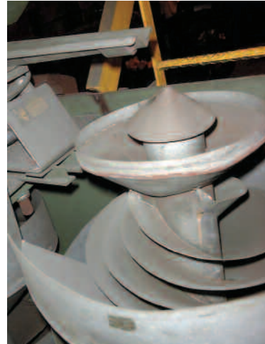
FIGURE 11-4 Spiral Separation System for Shot Media Classification
